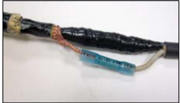
Connect the copper strands and the white wire with a connector and crimp.
