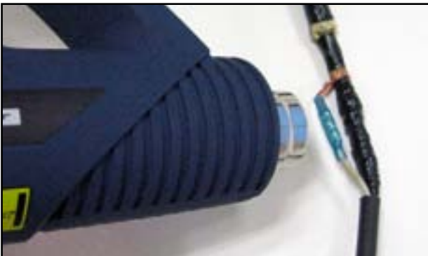
Cover with a tube and heat-shrink. Tape as before (pic 11).
