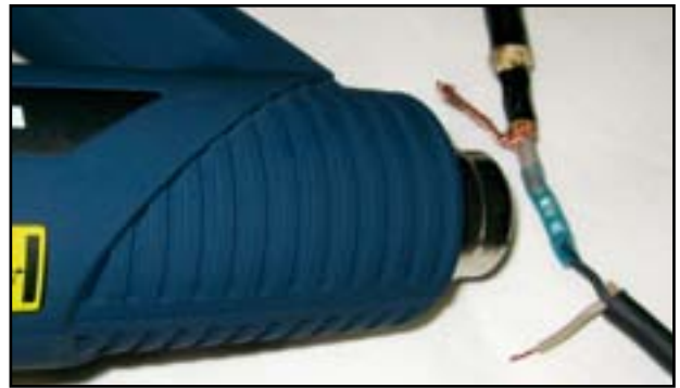
Fix the black wire of the connector cable to the connector, crimp and heat-shrink the tube into place.
