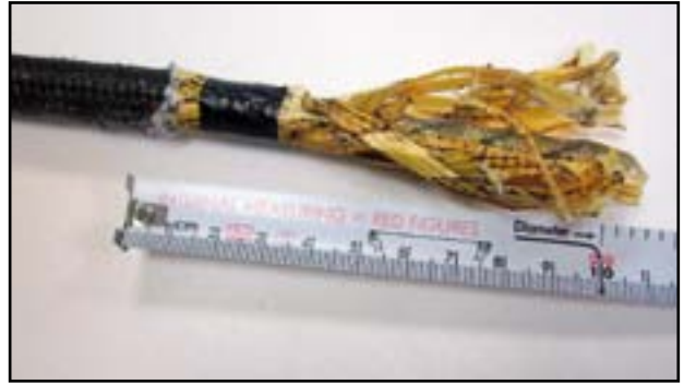
2 Glue the top 3cm of the braid and unravel 7cm of the Dynlce braid.
