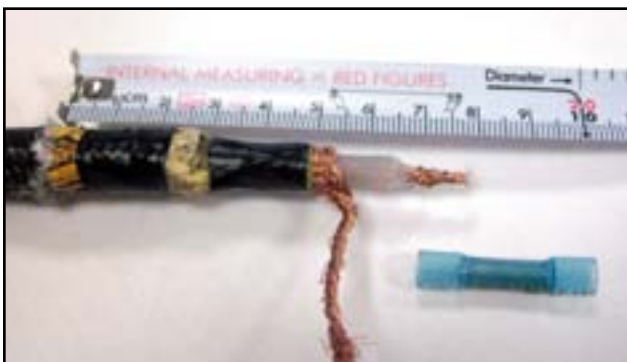
7 Shorten the conductor core so that it fits the connector.
