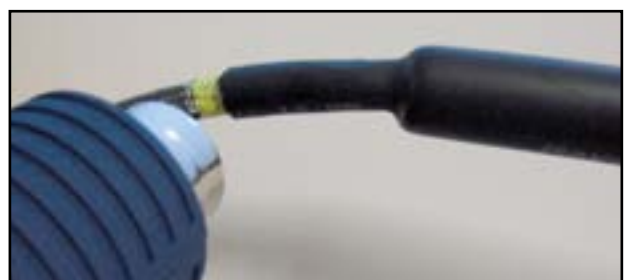
Shrink with a heat gun until it is tight over the connection.
