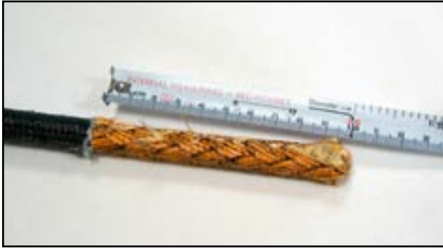
1 Cut away 10cm of the braided jacket from the end of the cable.
