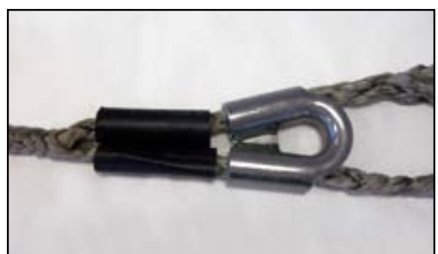
5 Slide the 10cm sleeves and the tube thimble onto the braids.
