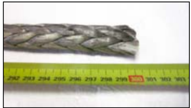
1 Measure and cut a 3 metre length of 14mm Dynlce 75 rope for the connector.
